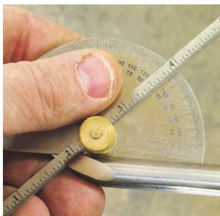
▲ Pic.2 If you are going to use the tool only for pull cutting, I would have the cutting angle at around the 55° mark. However, this would make it less efficient at push cutting, so I recommend grinding it to about 45° as a compromise
